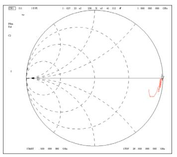
▲ Figure 4. The Smith chart, now displaying capacitance rather than inductance, when the offset is in place.
