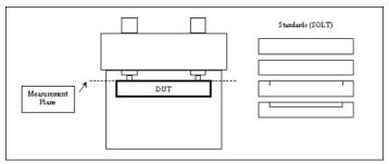
▲ Figure 1(a). A bandpass filter test fixture.
