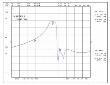
▲ Figure 8(b). The responses in 8(a) were significantly improved using the new calibration kit definition (b).
