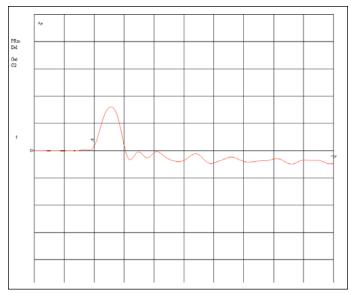
▲ Figure 7(a). In the time domain mode, the start and stop points of the gate are placed so that the fixture is removed from the measurement.
