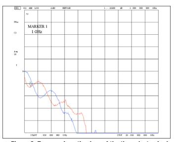
▲ Figure 6. Two-way insertion loss of the through standard.
