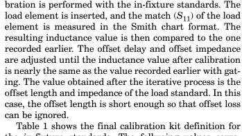
Table 1 shows the final calibration kit definition for the in-fixture standards. The following values correspond to a definition for an ideal calibration kit:
