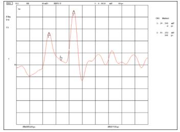
▲ Figure 5. Offset impedance, identified with markers between the two pogo-connector transitions.
